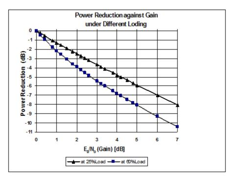
Figure (2) Power Reduction and Gain with Smart Antenna under Different Loading Scenarios
