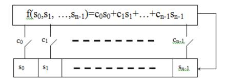
Figure (2) : Linear feed back shift register
