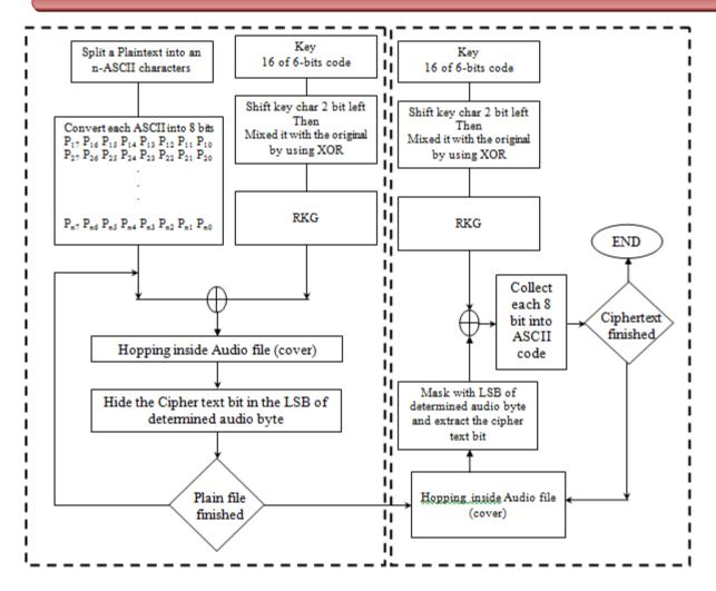
Figure (6) The block diagram of proposed system
