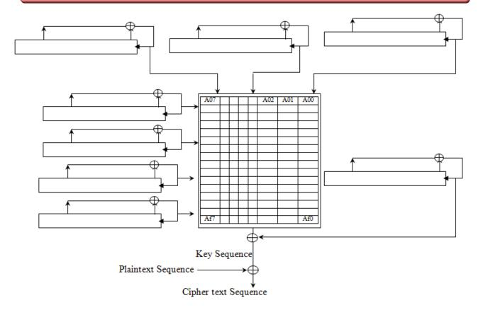
Figure (4) Cryptographic mechanism
