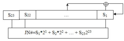
Figure (5).: The jumps mechanism
